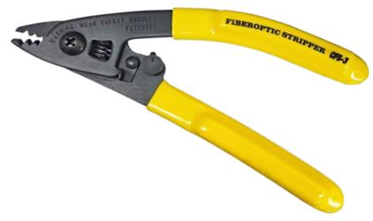
Three Hole Optical Fiber Stripper contains 3 holes, for stripping 250µm coated fiber and 900µm buffer tube. In addition, a 3rd hole for stripping 3mm fiber jackets. TK3 is a precision fiber tool, CNC drilled and made to exacting specification to allow the operator easily & efficiently perform daily fiber installation and maintenance tasks.
